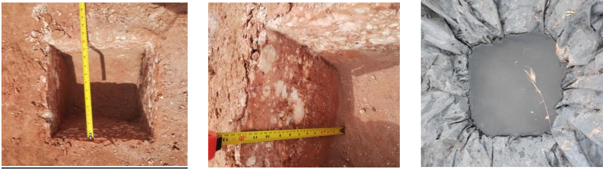
Figure 10-2: Pictures of the methodology for density estimation used for weathered rock.
