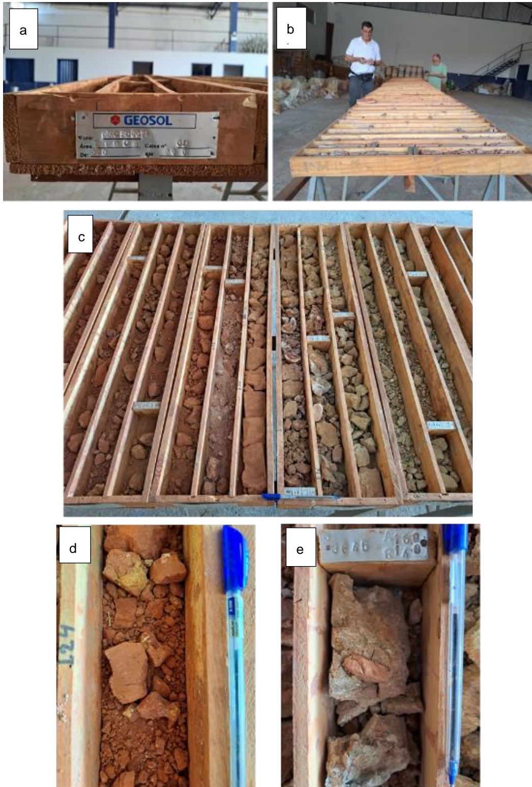
Figure 12-2: Diamond drill hole PMC-FD-0074: a) and b) Diamond drill hole PMC-FD-0074 core boxes; c) SOX zone on the left and MOX zone on the right; d) SOX zone detail; e) MOX zone detail.
