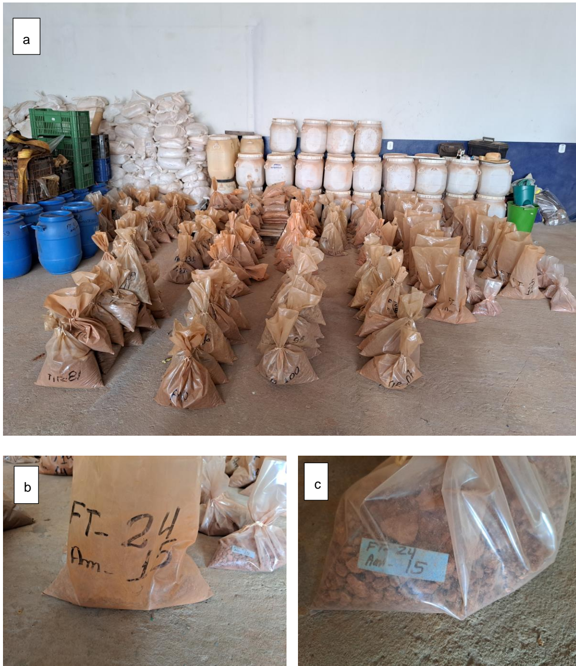
Figure 12-3: Auger drill holes: a) arrangement of samples in the drilling shed separated by hole; b) sample ID on the outside of the plastic bag; c) sample ID on the inside of the plastic bag.
