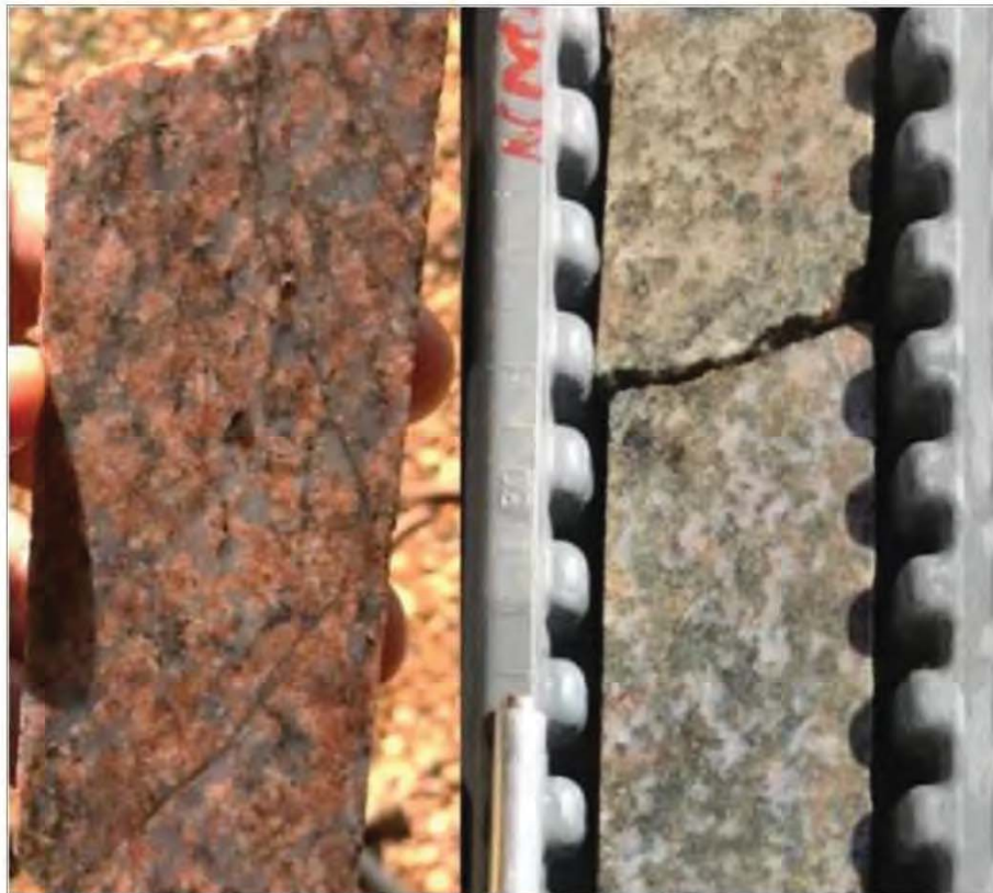
Figure 10-3: Hole NMDD-002 (left) host rock of monzogranite with some potassification and fine veinlets of chlorite and quartz; (right) main zone with strong sericite (chlorite) and intense sulphide dissemination.
