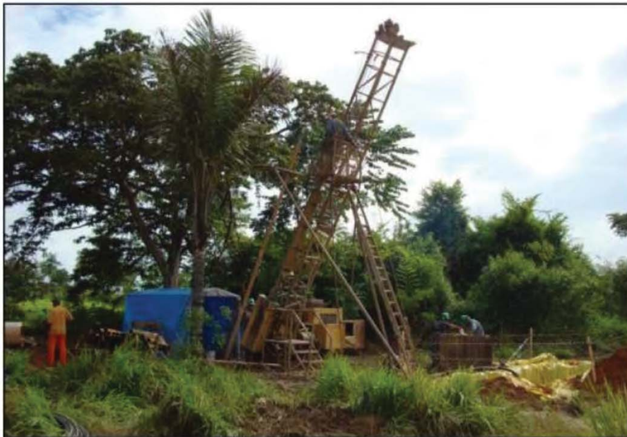
Figure 5-26: Diamond drilling operation by GMS – hole FD-DN 06 – area Raimunda
