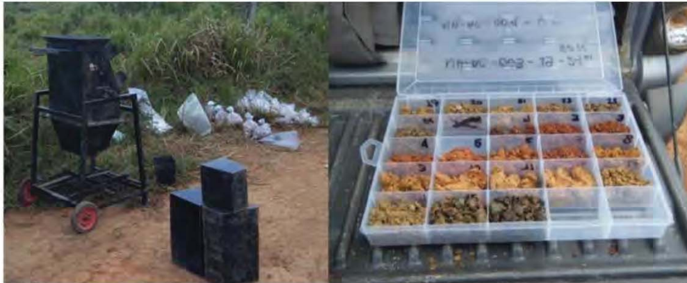
Figure 5-34: Left – the riffle splitter used to collect sub sample, Right – the 1m chip trays used for archiving
