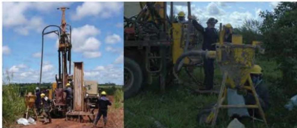
Figure 5-33: Left – the Sanvik KL150 AC drilling rock, Right – Cyclone used to collect the sample
