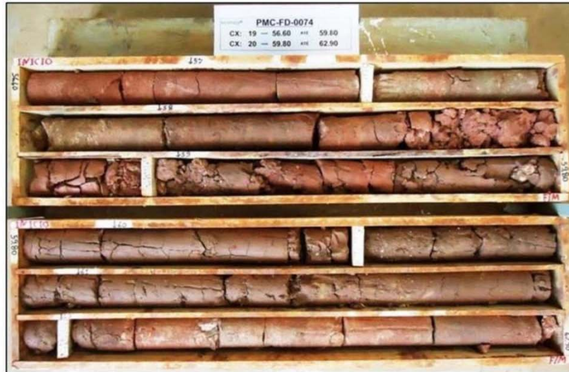
Figure 6-6 – Drilling core from borehole PMC-FD-0074 showing magnetic conglomerate from the Capacete Formation
