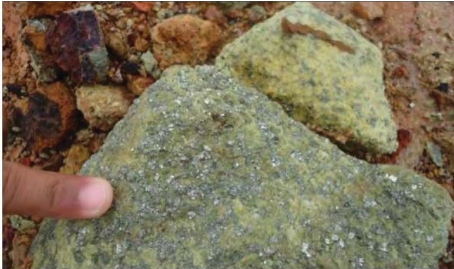
Figure 6-10: Photographs of a typical granite hydrothermalized and mineralized with disseminated pyrite (Luisão 01 pit)
