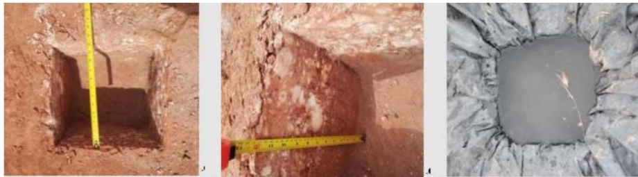
Figure 9-2 – Pictures of the methodology for density estimation used for weathered rock
